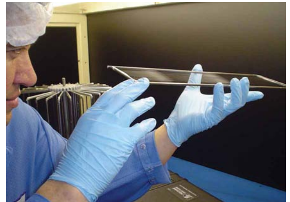
The coating must be uniform and free from surface defects.
