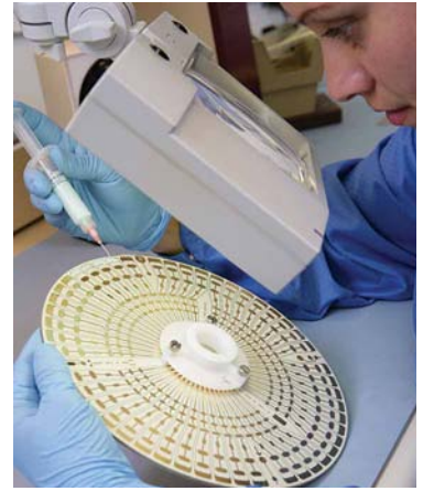
With proper masking, Parylene coating can be selectively applied to complex substrates.
